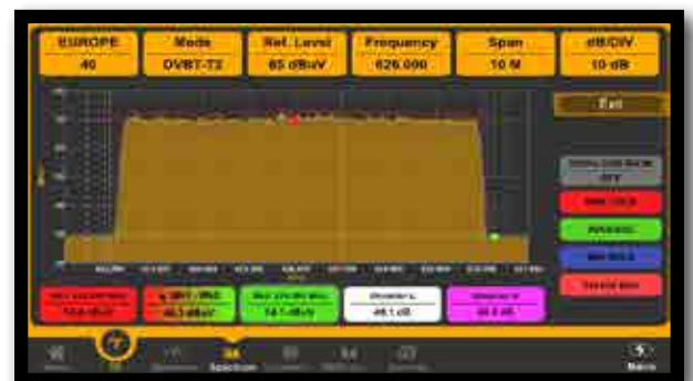
MARKERS, MAX and MIN HOLD, AVERAGE, SHOULDER MASK SX and DX CONFIGURATION EXAMPLE
