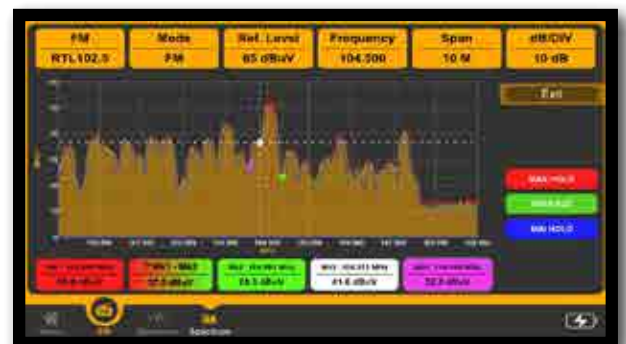
MARKERS, MAX and MIN HOLD, AVERAGE, SHOULDER SX and DX CONFIGURATION EXAMPLE
